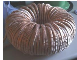
Figure 3: 3D model of a 1 st stage filter coil in the transmission path. The used litz wire contains 10000 strands with 63 \mu m diameter.
