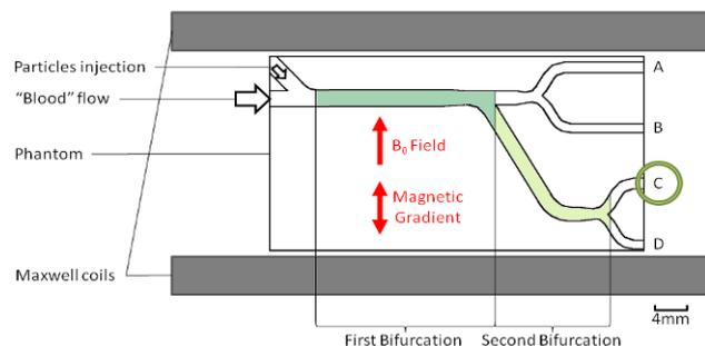
**Fig 1:** Experimental setup showing a phantom, with three Y-shaped bifurcations, inside the Maxwell coils. The targeted branch during the test was the C one.
