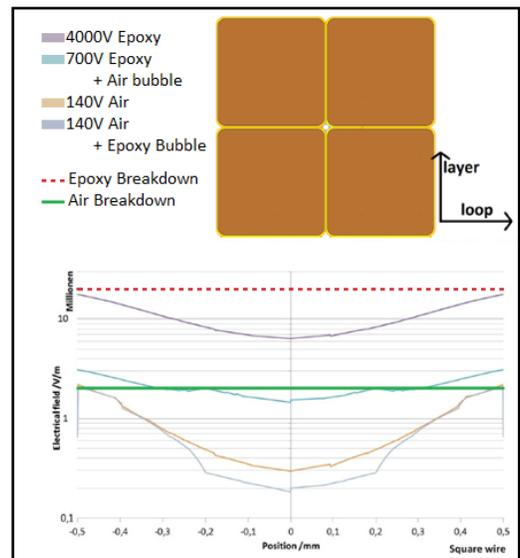
Figure 2. Electrical field and breakdown voltage between two layers of a coil made with a square Litz wire with a side of 7.3 mm. The material between the 4 wire changes between air and epoxy with and without a 0.4 mm bubble in the middle. The voltage difference is applied between the top and the bottom layer.
