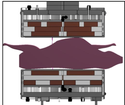
Figure 1. Cross section view of the scanner containing a mini-pig.
